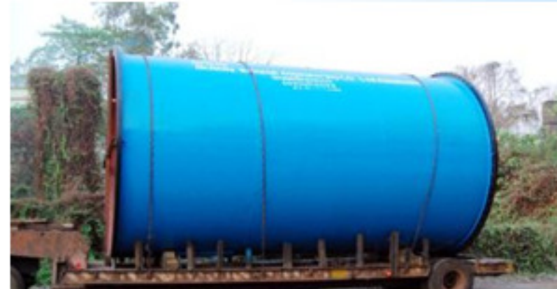
BALL MILL SHELL 4.8 m Dia X 8.0 m LG (FOR DEIFY)
